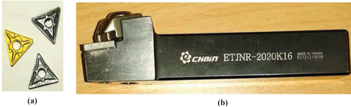
FIGURE 1. Cutting tools used in the study, (a) Carbide insert cutting tool, (b) Cutting tool handle
